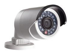
The 1.3 MP IP mini-bullet camera for outdoor use is a budget fixed-lens camera that produces 1280 x 960 output in low illumination with IR LED range to 30m. Features include PoE, a 4mm fixed lens, and a vandal-resistant housing.
