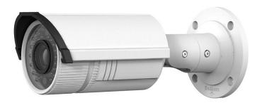
The 1.3 MP bullet is a mainline IP camera for outdoor use. Capable of 1280 x 960 resolution, the camera features PoE, a varifocal lens, and IR LEDs for nighttime vision up to 20m. Also included are audio and alarm I/O and a micro SD slot for up to 32 GB local memory.
