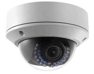
The Mainline 3MP dome is a high-resolution IP camera that is an appropriate choice for outdoor applications where image detail and/or wide coverage is important. Capable of 2048 x1536 resolution, the camera features a varifocal lens and 20 meter IR LEDs for use in low light conditions. The PoE camera includes a micro SD slot for up to 32GB local memory and is encased in a vandal-resistant housing.
