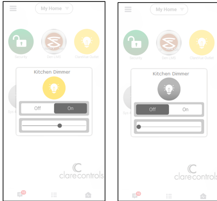
Figure 2: Dimmer at 60% and off
