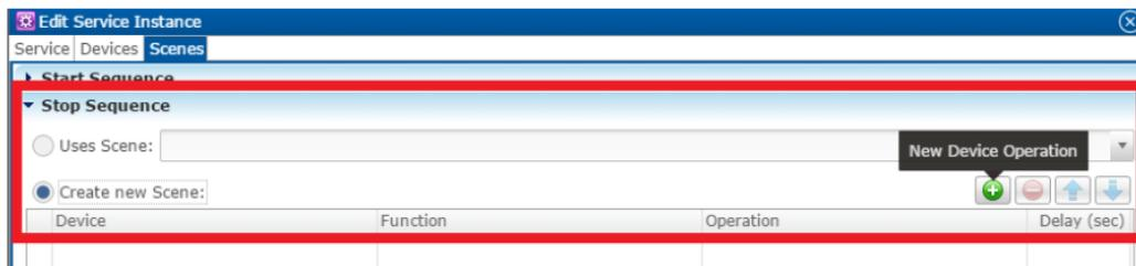
5. Configure the Device, Function, and Operation drop-down menus with the desired values.
