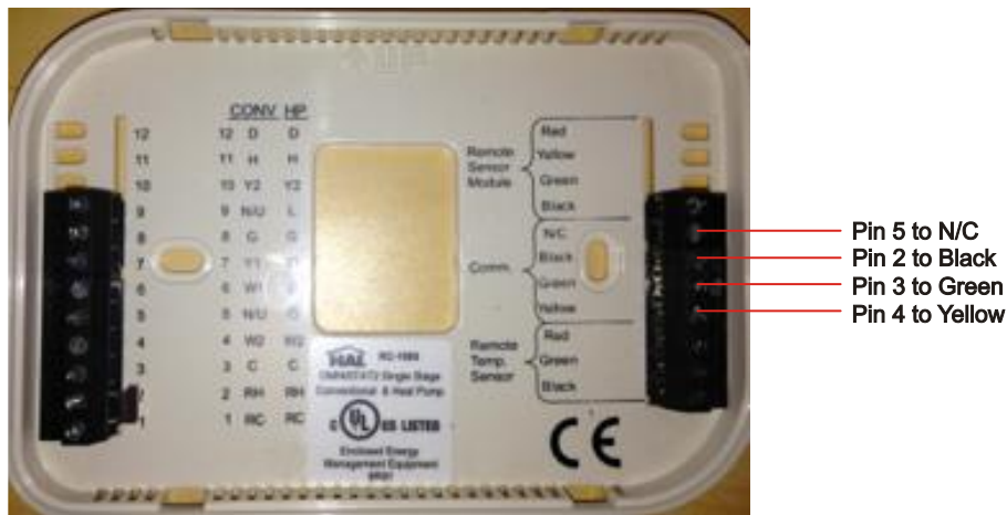
Figure 4: RC-2000 thermostat pin connections
