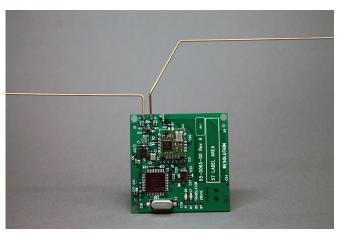
The Clare Wireless to Wireless Translator Module can be placed in Slot 3. The card enables system compatibility with Honeywell, 2GIG, GE, Napco & DSC sensors.
