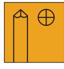
**Diamond Point** General purpose point with best holding power Blunt Diamond Point Effective at reducing wood splitting in hardwood applications
