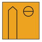
**Blunt Chisel Point** Effective at reducing wood splitting in hardwood applications
