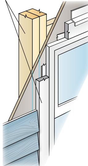
Notch plank around window trim and flashing.
