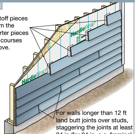
For walls longer than 12 ft land butt joints over studs, staggering the joints at least 24 in (for 24 in. o.c. framing) or 32 in. (two stud bays for 16 in. o.c. framing).
