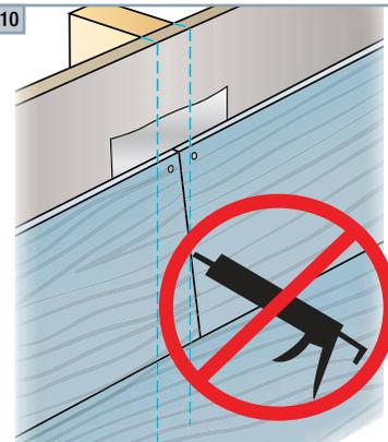
Caulking at HardiePlank lap siding butt joints is not recommended for ColorPlus for aesthetic reasons as the caulking and ColorPlus will weather differently. For the same reason, do not caulk exposed nail heads. Refer to the ColorPlus touch-up section for details
