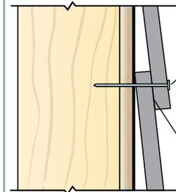
Exposed fasteners are driven through the face of the boards.
