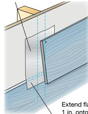
Extend flashing 1 in. onto the course below
