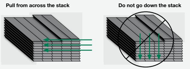
**TIP:** When taking planks from the pallet installation, avoid repeating the texture pattern by working across the pallet. Two to four planks can be removed from a stack at one time. But then material should be taken from adjacent stacks, again working across the pallet. Texture repeat is typically a concern on large walls with few breaks such as windows or doors.
