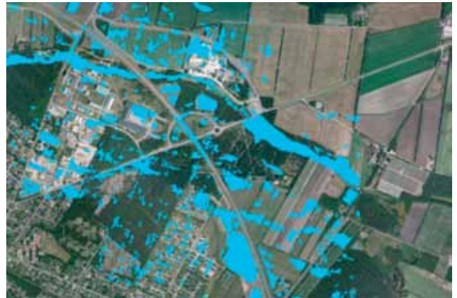
Screening of terrain data (identification of 'blue spots')
