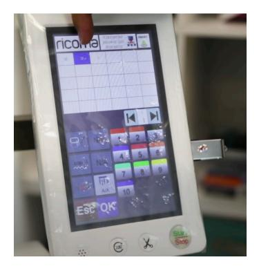
Go to colors and select the "frame out" option for the first 2 steps. This will tell the machine to frame out the design so that you're able to then attach the straps.
