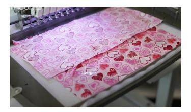
Place your two new strips of fabric on top of your mask with the design facing down. Make sure they are covering the mask completely and that they are overlapping each other.
