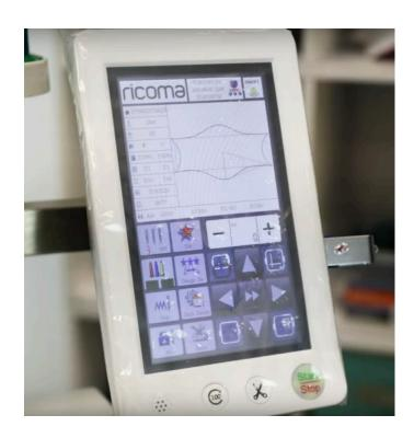
Download the .DST file to your machine and choose a hoop size based on the size of the mask and the design.
