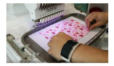
Place the main fabric on top of the trace stitch with the design facing up and press start.
