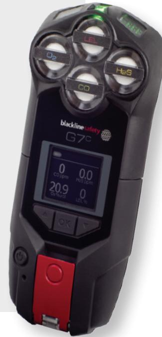
Following a successful evaluation, the G7/Beacon system from Blackline Safety was deployed across the site. Users were already carrying rented 4-gas detectors, so Osborne were able to utilise the rental budget to swap the previous devices for G7s providing increased safety to the teams.
