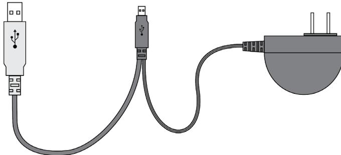
3. Connect the three-ended firmware installation cable into their respective ports. Plug the USB into the USB port on your computer, the micro USB into Blackline device, and the wall charger into a power outlet.
