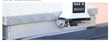
G7 Bridge can be mounted to a truck bed tool box if it has an unobstructed line of sight to the sky. Screw the multi-purpose mount to the G7 Bridge Mounting Bracket plate, and screw the plate to the side of the tool box. Slide and snap G7 Bridge into the multi-purpose mount, and lock G7 Bridge Mounting Bracket with key for additional security. Ensure the LCD screen is facing outwards for operation.
