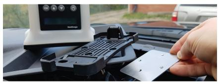
Remove the dash tray or portion of the dash you want to mount to. Screw the multipurpose mount to the top of the dash, then screw the dash plate under the dash tray to secure the mount in place. This is best suited for a Ford F-150 with removable dash tray to avoid drilling directly into vehicle dashboard.
