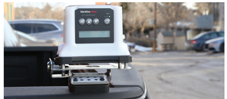
Bridge mounted to the anchor points on a truck bed rail pop-out
