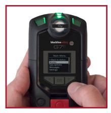
Use the down arrow to scroll down to the "modes" option, and press OK to select it.
