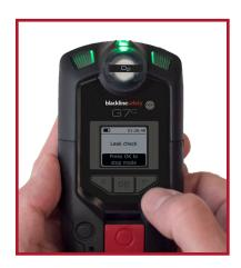
The current mode can be checked at any time by pressing the down arrow while on the gas status screen. Configuration modes can also be changed from this screen by pressing OK.
