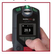
Press OK to wake up G7's gas status screen, and press it again to access the main menu.
