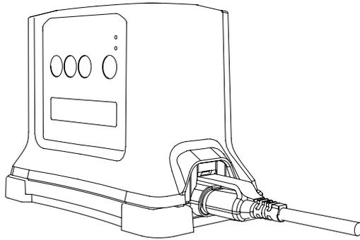
VDC power without splicing into the vehicle's electrical system. Installation instructions accompany the fuse expander accessory, when purchased. Two sizes of fuse expander are available: Mini and ATO. Contact Blackline for more information.
