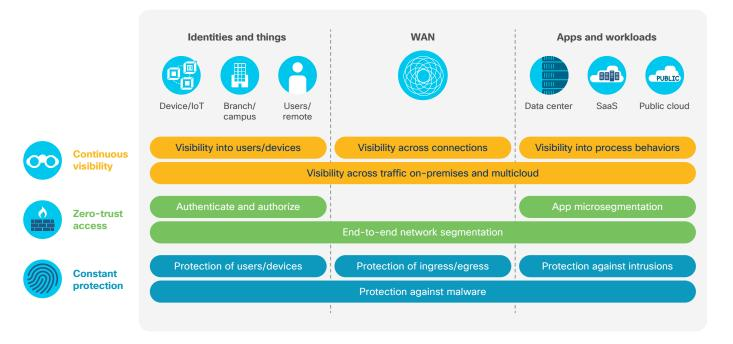
A full view across access, WAN, data center, multicloud, and IoT networks allows the mapping of every flow that traverses the network so that teams can determine a dynamic baseline of normal network behavior. With an intelligent network that provides full visibility, the network team has an invaluable resource to help the security team detect and remediate threats faster and more accurately—even in encrypted traffic.
