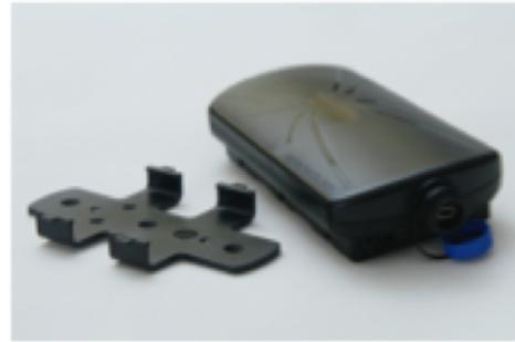
Secure the spider to the dashboard with the bracket supplied. The spider unit can be quickly removed from the mount when required. The top of the spider must point up. The Spider is not subject to Specific Absorption Rate testing, however we recommend placing no less than 200mm from a person.
