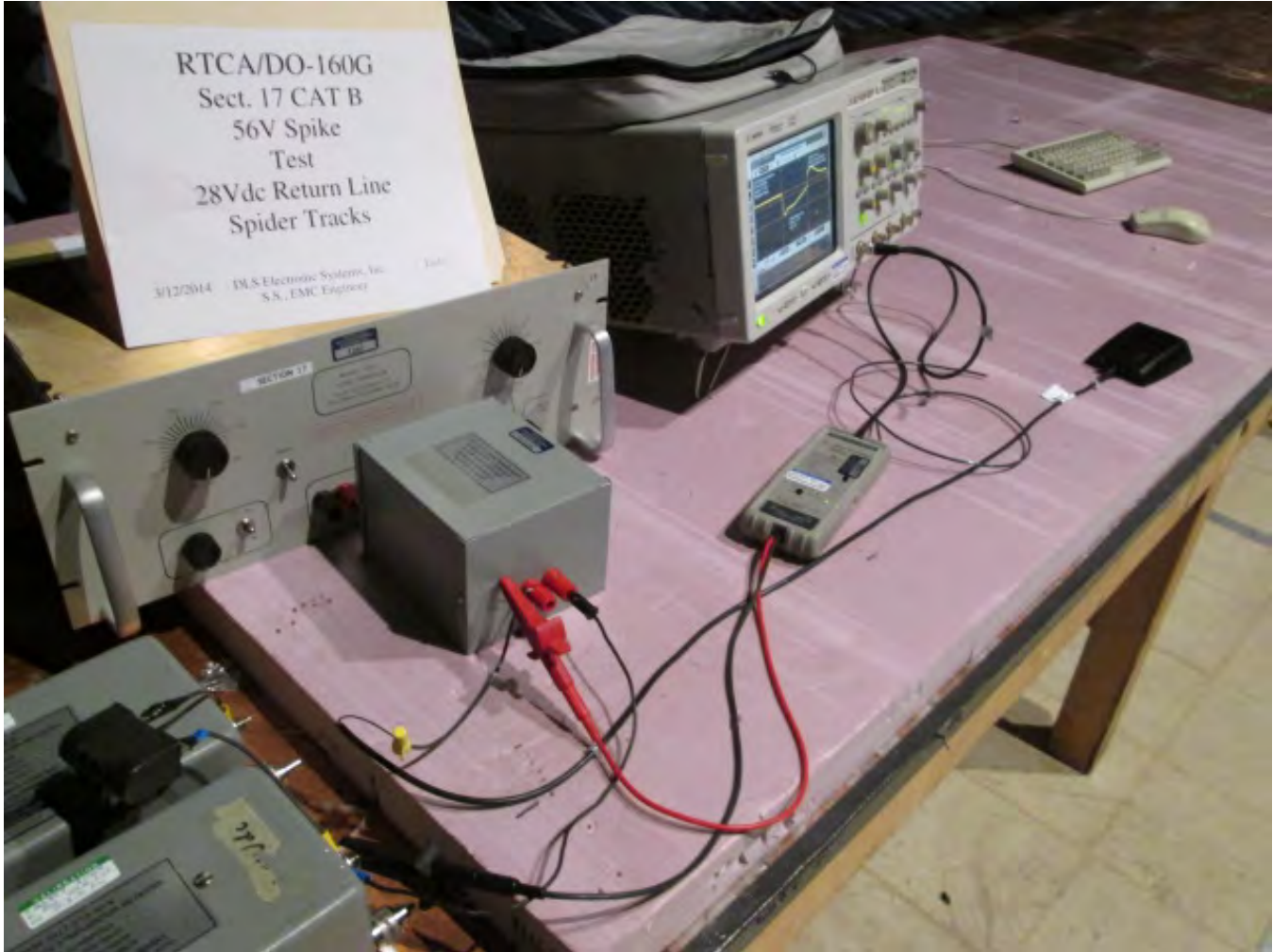
Section 17 Test 28 Vdc Return Line
