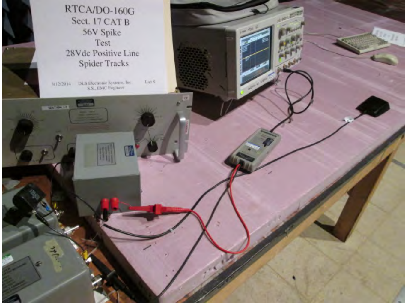
Section 17 Test 28 Vdc Positive Line
