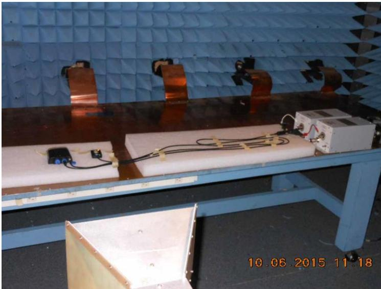
Section 21.5 - HF Horn Antenna, 1 - 6GHz, Vertical Polarization
