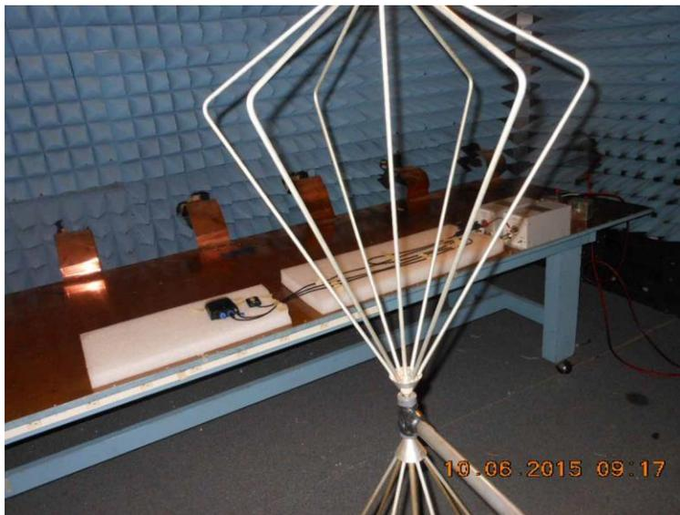
Section 21.5 - Bicon Antenna, 100 - 200MHz, Vertical Polarization
