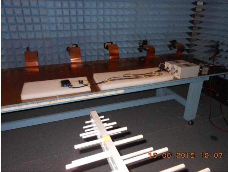
Section 21.5 - Log Antenna, 200MHz - 1GHz, Horizontal Polarization
