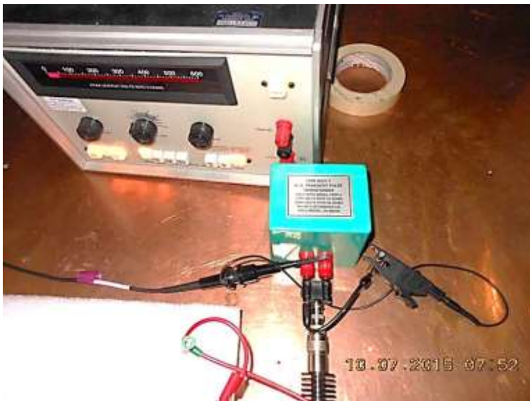
Section 17 – Calibration Setup, 50 Ohm
