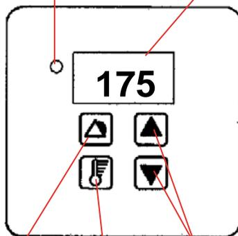
Alarm Reset Button      Temperature Set Button      Up and Down Arrow Buttons
