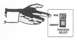
e. If you are not ready to cook, place the FUNCTION SWITCH in the SIMMER position. This will cause the heating element to shut off and the internal thermostat to maintain the water temperature at around 205°F.
