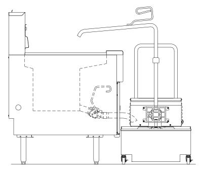
bottom of the fry pot. When the fry pot is clear close drain valve and return all of the oil.
