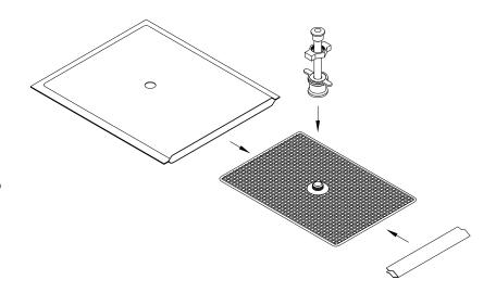
Sprinkle filter powder over filter envelope assembly, if desired.
