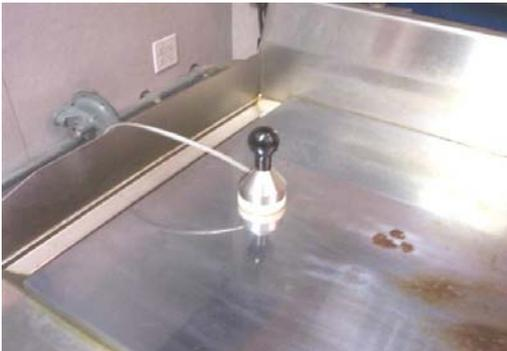
Place a weighted griddle temperature probe on the cooking surface 9-12" from the front edge of the griddle plate.
