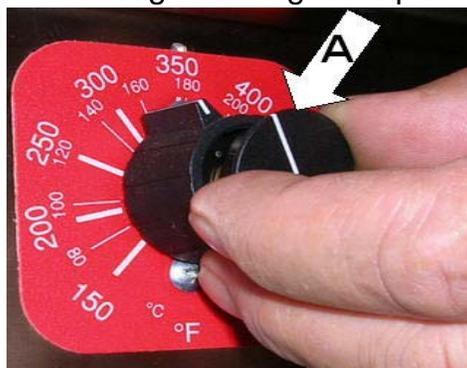
While the Unit stabilizes at Temperature for 30-60 minutes, remove the control knob caps
