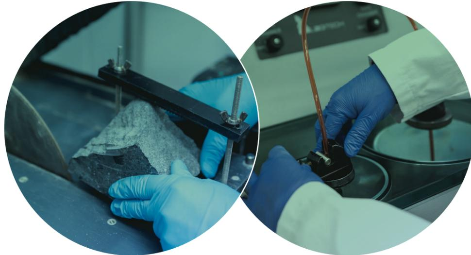
**GTS1 thin section cut-off & trim saw**
