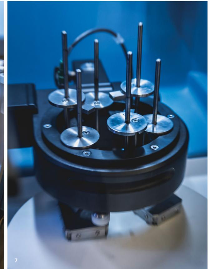
In addition to standard thin and ultra-thin section production, Logitech systems are versatile enough to accommodate material requiring special processing techniques such as concretes, fluid inclusions, coals and soils. Non-geological materials such as bone implants and tooth are also catered for.
