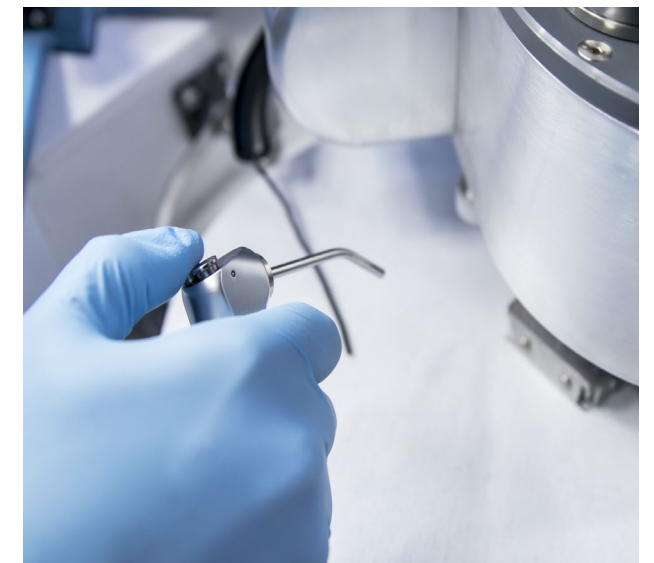
IN-SITU SAMPLE CLEANING WITH INTEGRATED DI WATER AND NITROGEN GUN
