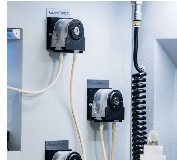
METERED ABRASIVE FEED VIA PERISTALTIC PUMPS
