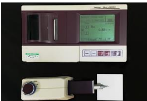
Above: the Mitutoyo SJ400 measures roughness on a substrate.
