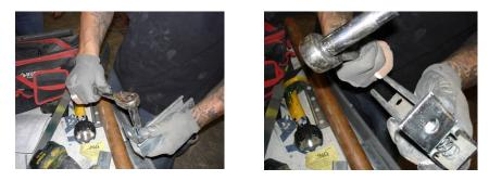
Why the incident occurred: The socket slipped when he was tightening the bolt causing his right finger to hit the Unistrut. The piece of Unistrut was not deburred after being cut. The result: Three hours in the clinic and eight stitches.
