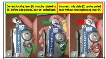
Proper operation of the sleeve is shown in green above. The locking lever (A) must be rotated to position (B) for the side plate (C) to be pulled backwards. If your sleeve functions in this manner, it is working properly. If you are able to pull the side plate (C) back by pulling on the top roller without first rotating lever (A) to position (B), then the unit should be removed from service (see red example above).
