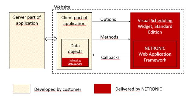
All required objects are defined and identified within this FDD. These objects, the functions and the callbacks are part of a custom application programming interface (API) that can be addressed via interface.
