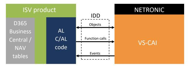
All required objects for the VS-CAI are defined and identified within the IDD. These objects, the functions and the events are part of a custom application programming interface (API) that can be addressed in Dynamics via AL code or C/AL code, respectively.
