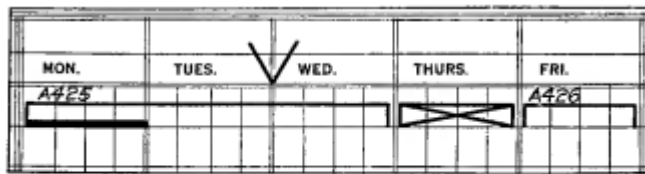
FIGURE 18. HOW WORK BEHIND SCHEDULE IS SHOWN BY THE GANTT LAYOUT CHART
