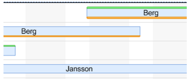
TWO LAYERS INDICATING PROBLEMS OR CONFLICTS; ONE LAYER ON TOP OF BAR AND ONE LAYER AT BOTTOM OF BAR
