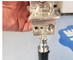
Figure 6: Threaded end on Stand & Mounting Block Holes
