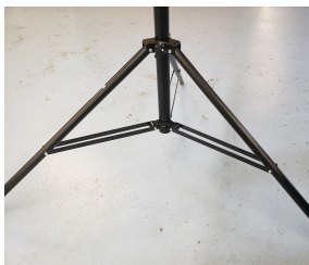
Figure 3: Correct Cross Bar Orientation
