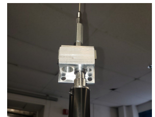
Figure 7: Mounting block screwed onto Stand
