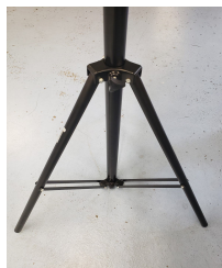
Figure 4: Incorrect Cross Bar Orientation
