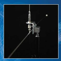
The RF Venue FM Antenna uses an orthogonal ground plane that preserves bandwidth and very low SWR over the entire FM band without tuning. It is rated for 10 mW to 100W continuous operation. A low wind load antenna element and ground plane element are suitable in outdoor locations where there may be wind present, and the supplied user-filled sandbag easily clips to the base via a supplied carabiner to reduce or eliminate tipping.
