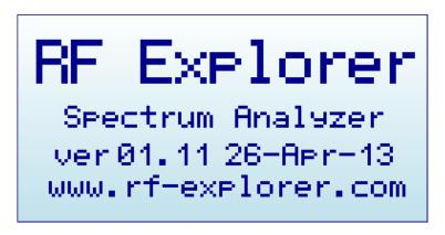
**Note**: if you enable this screen for more than 30 seconds while connected to USB port and power switch in the unit set to ON, RackPRO will automatically go to low power mode and will switch the LCD off, but will keep charging the battery. This is suggested when you intent to charge the internal battery but not make use of the unit for measurement.
