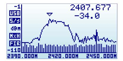
The X axis represents frequency in MHZ and Y axis display actual received power in dBm or dBuV (selectable).
