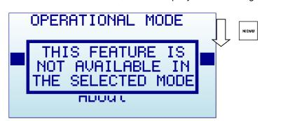
If your analyzer includes two modules (e.g. ISM Combo) only one of the modules may be the one with the available functionality. Make sure to select the right module before trying to use the functionality (e.g. the ISM Combo has the 2.4G module enabled on the SMA module at the right) otherwise above message will popup.
