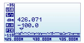
**Note**: While RackPRO Spectrum Analyzer screen is enabled, the [Left] and [Right] buttons can be used to increase or decrease the Start/Stop frequency, virtually moving the visible spectrum
