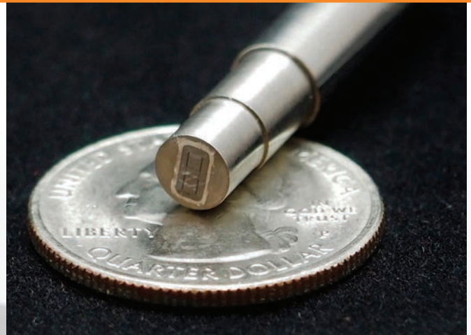
Optical gratings on a micromachined floating element enable direct measurement of shear stress in harsh environments
