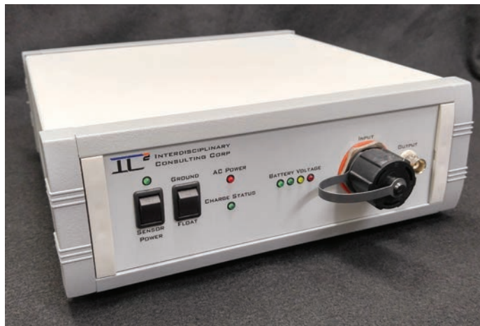
The SCU provides a fiber-coupled optical source and detectors and electronics to produce an analog voltage for output to a DAQ
