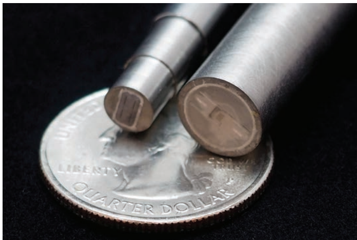
Micromachined floating element sensor heads comprised of Silicon/Pyrex (left) and Sapphire (right).
