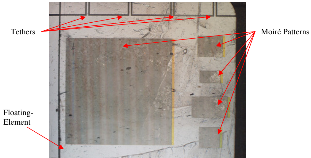
Figure 9: Photograph of the micro-fabricated floating element in the optical test-bed that is used to simulate the Moiré sensor as viewed through the Pyrex layer.
