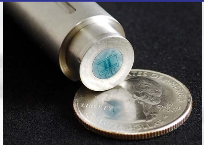
Micromachined sensor heads in stainless steel housings for flush-mounted installation
