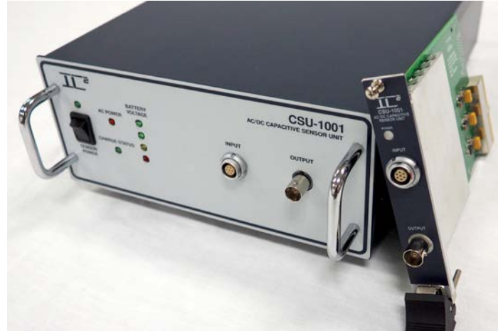
The SCU provides low-noise power and bias voltages to the sensor head and conditions the analog voltage signal for output to a DAQ
