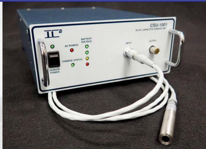
Complete sensor systems for non-intrusive, direct, simultaneous mean and fluctuating wall shear stress measurement
