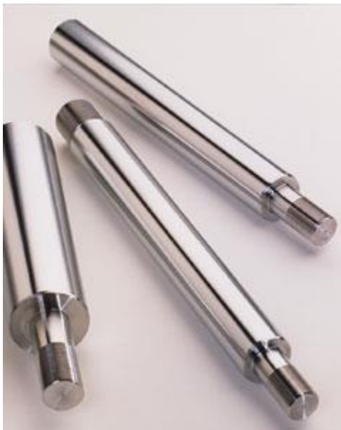
Piston rods to 3.5" (88.9-mm) OD are machined complete from chrome-plated bar on the Bardons & Oliver ISC 350 CNC lathe.
