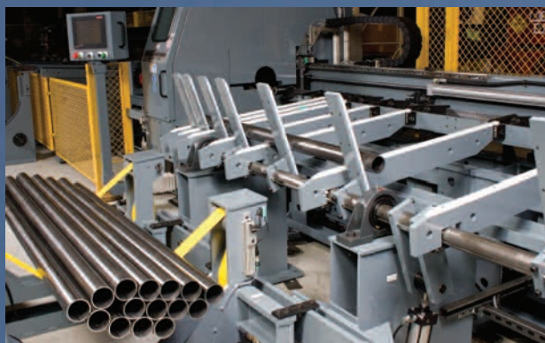
Unload parts without interrupting production. Buck-style unloader collects finished parts for bundling. Unloader holds back parts and allows production to continue.
