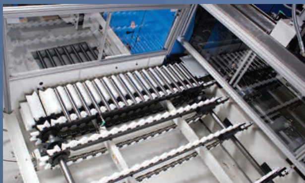
Protect finished parts from damage. Singulating unloader for parts made from chrome bar eliminates any risk of marking or scratching high precision parts.
