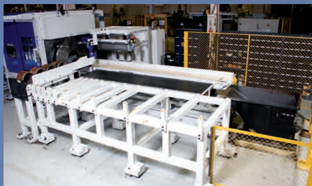
Unload a variety of finished parts. Combination unloaders handle high production of short blanks or long parts.
