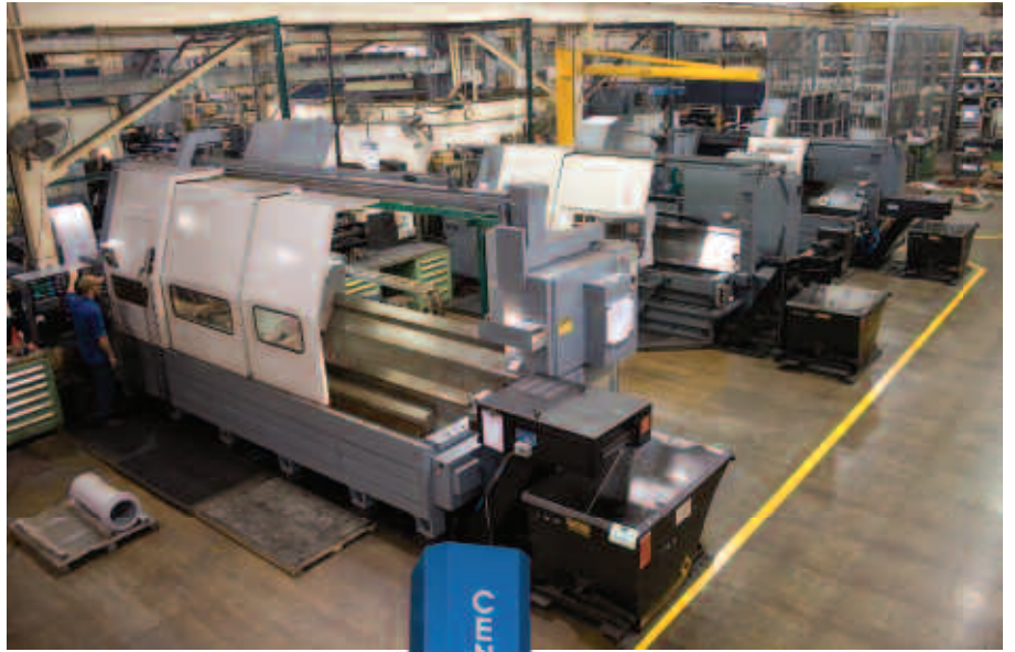
Horizontal turning capacity: up to 36" diameter and 144" long.
