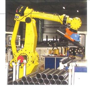
Bardons & Olivers' CNC machines. It can be retrofit to a customer's existing system, and its flexibility allows it to be integrated smoothly into a current setup. "The customer's material can be DOM steel tubing, seamless tubing and cast iron or steel bar stock," says Dalton. "The robot allows the parts to be picked up, drained of coolant, if necessary, and neatly stacked in a bundle buck for shipment or moved to the next operation sequence."
