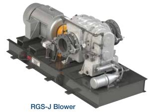
This is a Rotary Positive Displacement Gas Compressor with Integral lubrication to supply oil to the bearings, timing gears, and mechanical face seals. The Compressor is direct driven by an electric motor. The oil system includes a motor driven auxiliary oil pump in the forefront.
