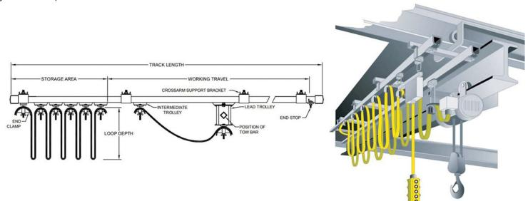
Festoon systems are extremely reliable and can be used in all kinds of applications from indoor to outdoor applications, high heat environments, and in other demanding environments like in mills and at port facilities. They can also be used to safely provide power and control for explosion proof cranes.
