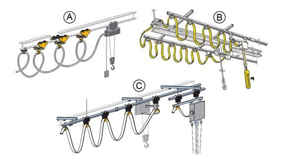
**Track-Mounted Cable Festoon Systems** – effective cable management in light to medium-duty applications. Trackmounted systems allow you to organize and move cables and/or hoses for power and control circuits. These systems are reliable, efficient, easy to install, and have low maintenance requirements.
