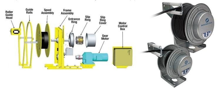
Cable reels utilize a very simple design that automatically winds and stores flexible cables. Cable reel electrification requires little to no maintenance and is easy to install. They can also be mounted stationary, or on a swivel base to allow the cable to payout in multiple angles and directions.
