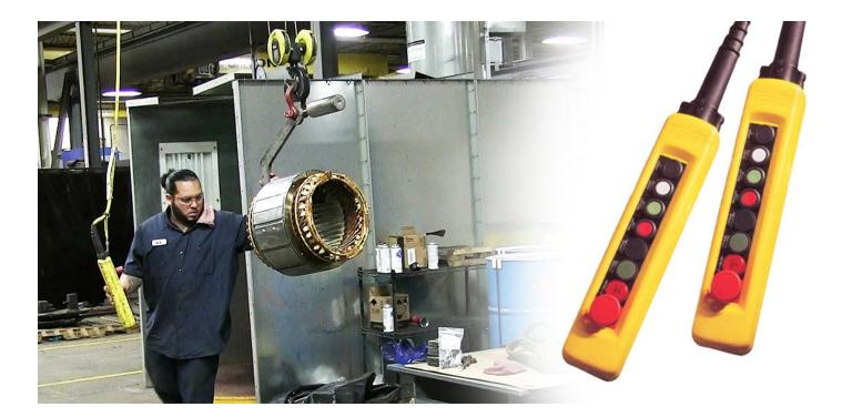
The operator can also laterally position the hoist and control the up and down lifting movement of the hook using the pendant control.
