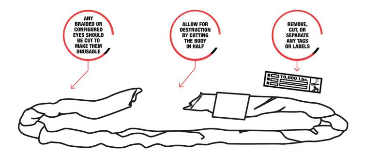
If it is determined that a roundsling meets the removal from service criteria, then the following actions need to be taken to discard and render the sling unusable:
