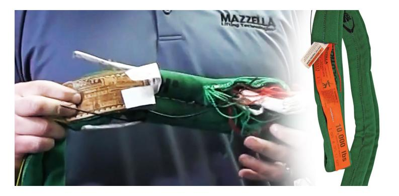
The following ASME B30.9 high performance roundsling inspection standards require immediate removal from service for any sling with any of the following visible occurrences:
