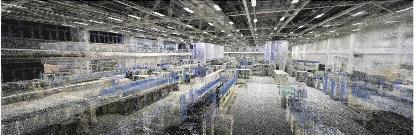
*Point cloud of the Siemens' factory scanned with the NavVis Indoor Mobile Mapping System M6*
