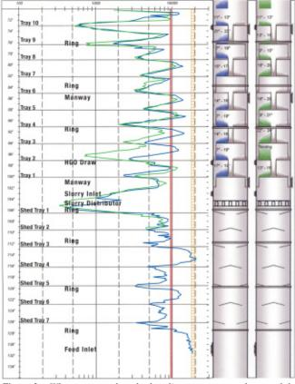
Figure 2 - When compared to the baseline scan a second scan of the Main Frationator indicated Trays 2 and 3 showed observable differences in the liquid level on these trays.
