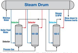
Figure 7 - Detector placement for TRACERCO Diagnostics<sup>TM</sup> Leak Study on a WHB.
