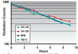
Figure 8 - Test results indicated that the 101-CB exchanger had a slower rate of decay.
