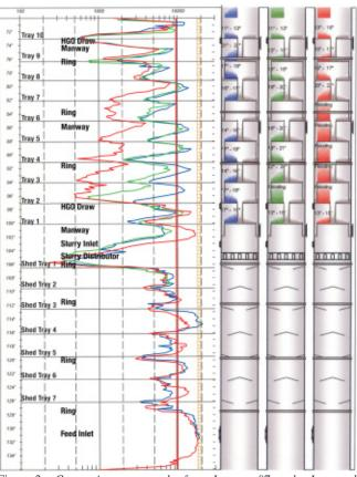
Figure 3 - Comparing scan results from January 07 to the June and December 06 scans indicated that flooding had increased from Tray 2 in June 06 to Trays 2 - 7.
