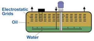
Illustration of **The TRACERCO Profiler**<sup>TM</sup> housed in dip-pipes and installed within a vessel through a single flange.
