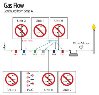
Figure 6 - Flow studies were performed through several portions of the flare line to isolate which unit contained a leak.
